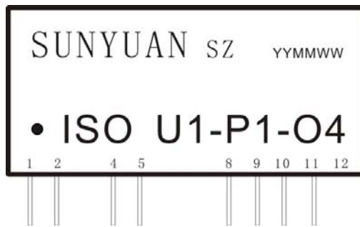
Voltage Signal Output Product PIN Diagram (0-2.5V/0-5V/0-10V)
