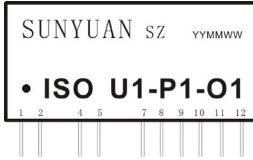
Current Signal Output Product PIN Diagram (4-20mA/0-10mA/0-20mA)
